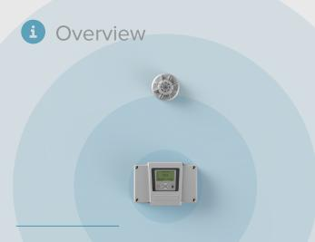
The Wi-Fyre Wireless A2R Heat Detector consists of a ProFyre ROR heat detector head combined with the Wi-Fyre wireless base. The ROR heat detector uses a thermistor arrangement to sense a quick rise in temperature and also a final threshold temperature of 57°C.
